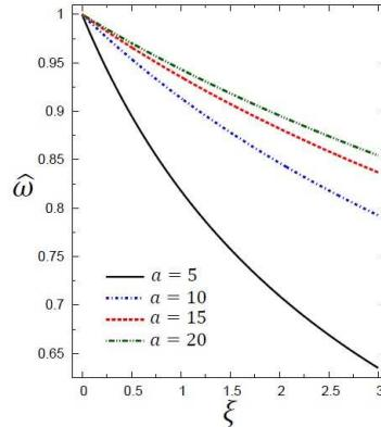
**Figure 2: Fundamental Frequency Ratio of a SLGS Vs Nonlocal Index and its Length ( $b = 10$  nm,  $h = 0.34$  nm,  $K_1 = 0$ ,  $K_2 = 0$ )**
