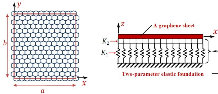
**Figure 1: A Continuum Plate Model of a Single-Layered Graphene Sheet Resting on Elastic Foundation**
