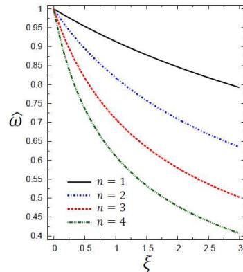
**Figure 3: Natural Frequency Ratio of a Square SLGS Vs Nonlocal Index ( $a = b = 10$  nm,  $h = 0.34$  nm,  $m = 1$ ,  $K_1 = 0$ ,  $K_2 = 0$ )**
