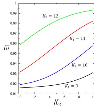
**Figure 6: Fundamental Frequency Ratio of a Square SLGS Vs Pasternak's Parameter ( $h = 0.34$  nm,  $a = b = 10$  nm,  $\xi = 1$ )**
