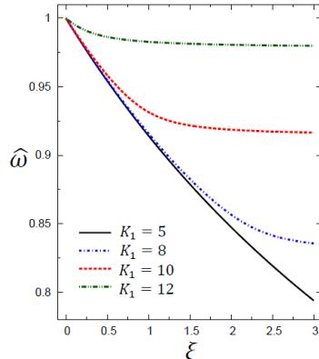
**Figure 4: Fundamental Frequency Ratio of a Square SLGS Vs Nonlocal Index and Winkler's Parameter ( $h = 0.34$  nm,  $a = b = 10$  nm,  $K_2 = 5$ )**
