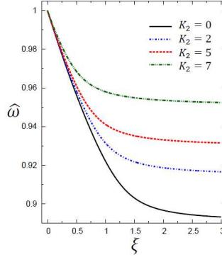
**Figure 5: Fundamental Frequency Ratio of a Square SLGS Vs Nonlocal Index and Pasternak's Parameter ( $h = 0.34$  nm,  $a = b = 10$  nm,  $K_1 = 10$ )**
