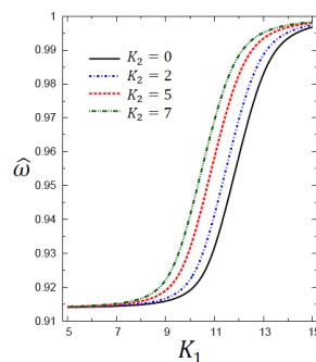
**Figure 7: Fundamental Frequency Ratio of a Square SLGS Vs Winkler's Parameter ( $h = 0.34$  Nm,  $a = b = 10$  Nm,  $\xi = 1$ )**
